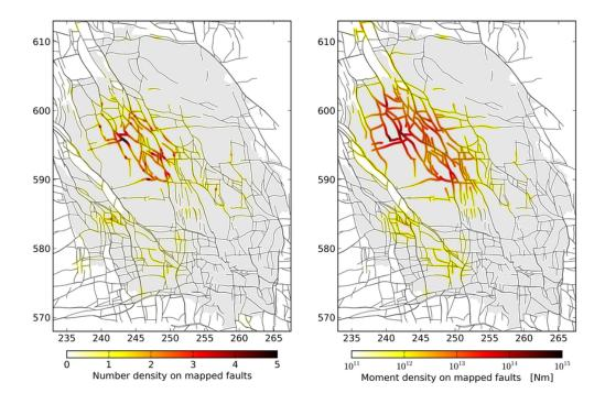
Figure 20: Estimates for the event number density (left) and the seismic moment density (right) obtained from the  $M \ge 1.5$  events observed between April 1995 and December 2013 conditional on every event originating on a mapped fault.
