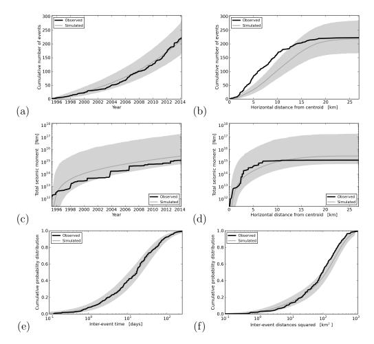
Figure 15: As Figure 9, except for the simulation results from the seismological model based on an exponential compaction trend Poisson process and an ETAS process. These simulations were based on Monte Carlo model parameter estimates. The dark grey line denotes the median simulation and the light grey band denotes the 95% confidence interval about the median.
