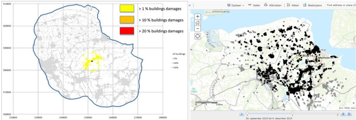
Figure 9.12 Prediction of chance of building damage using the TNO methodology (left) compared with actual damage claims (right) for the Hellum earthquake.
