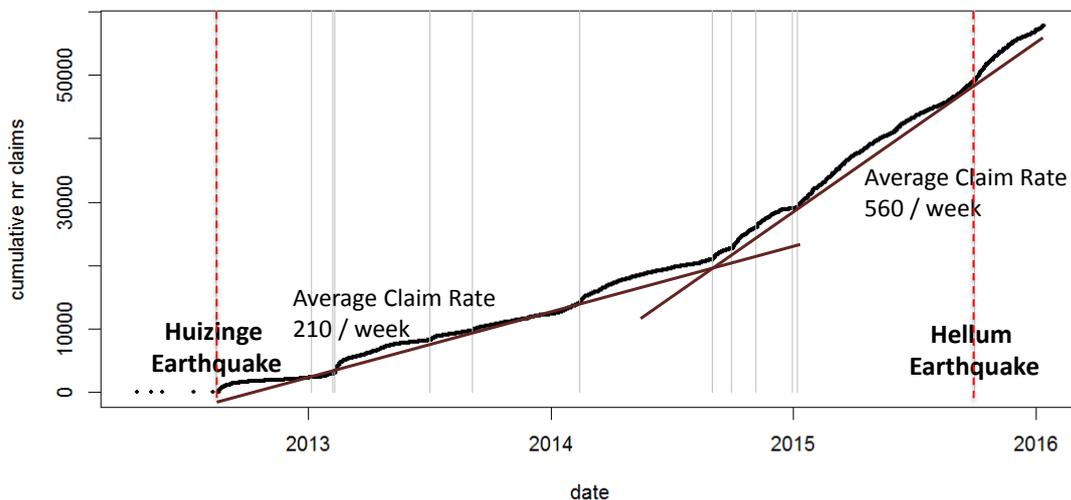
Figure 9.2 Cumulative number of damage claims over time.
