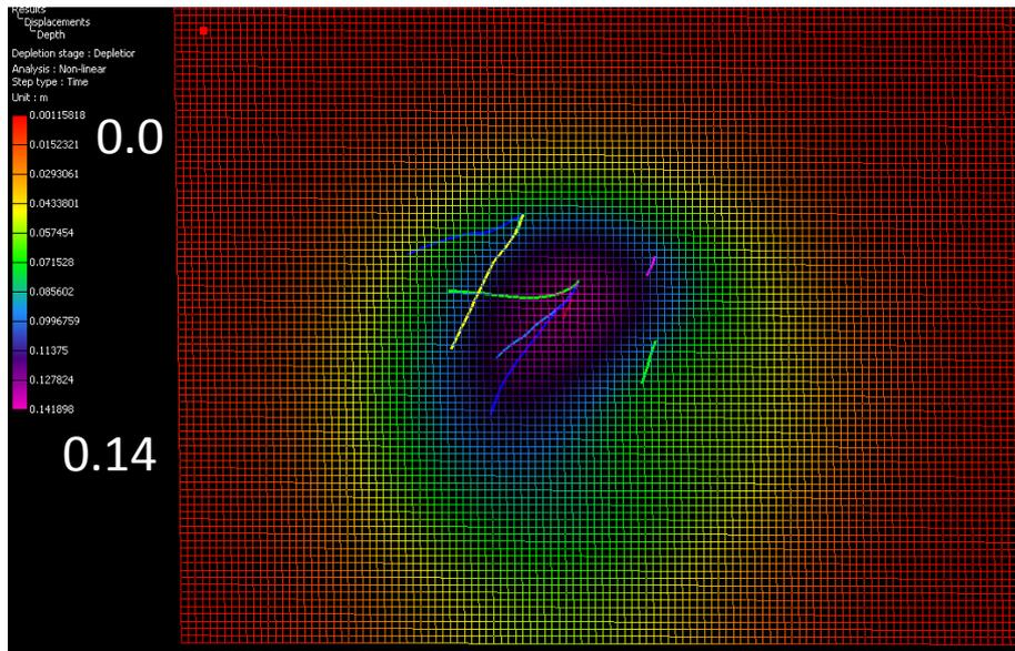
Figure 3.6: Subsidence bowl (0-14 cm) resulting from concentrated dissolution, also showing some well paths.
