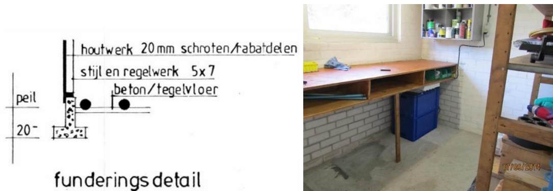
Figure 2.5a and b: Foundation detail of the shed
