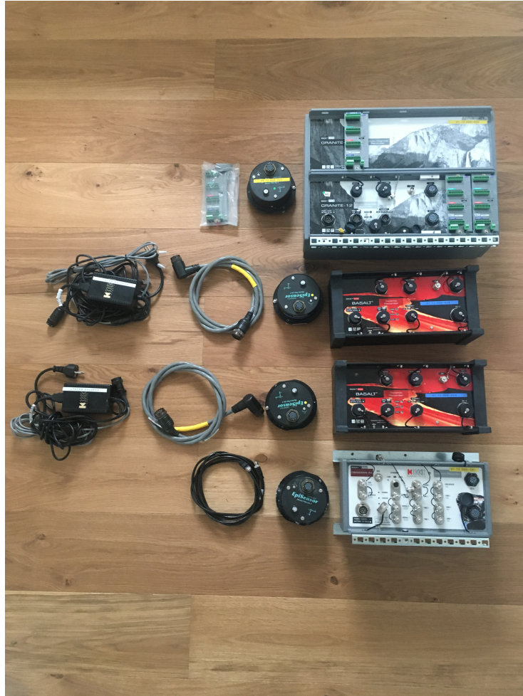
Figure 8. Sensors, cables and dataloggers removed from the 4 stations
