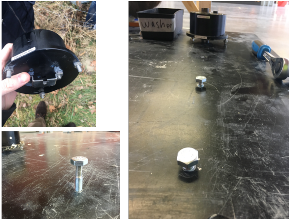
Figure 12. Mounting bolts modified from M10 for mounting the KNMI sensors on the table
