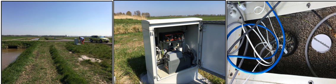
Station G39 Photos. Left: Overview of site. New VBB borehole accessory box is in foreground, G39 box in background ~30m distant. Middle: Inside G39 box, showing 14 channel Granite datalogger. Right: strong motion sensor located underneath the datalogger.
