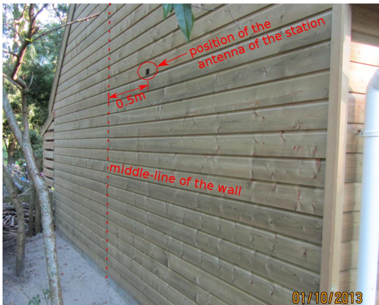
Figure I.1 Location of the antenna of the BOWW-station outside of the wooden shed
