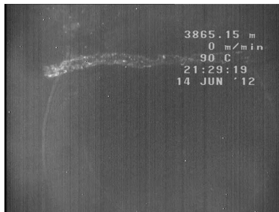
Figure 3: Video shot of the 11 ¾" connection at 3816 m
