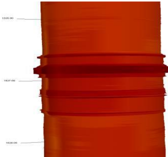
Figure C-3: 3D-caliper image of TUB-10 casing joint at 1827 mAHDF, Oct 2013.
