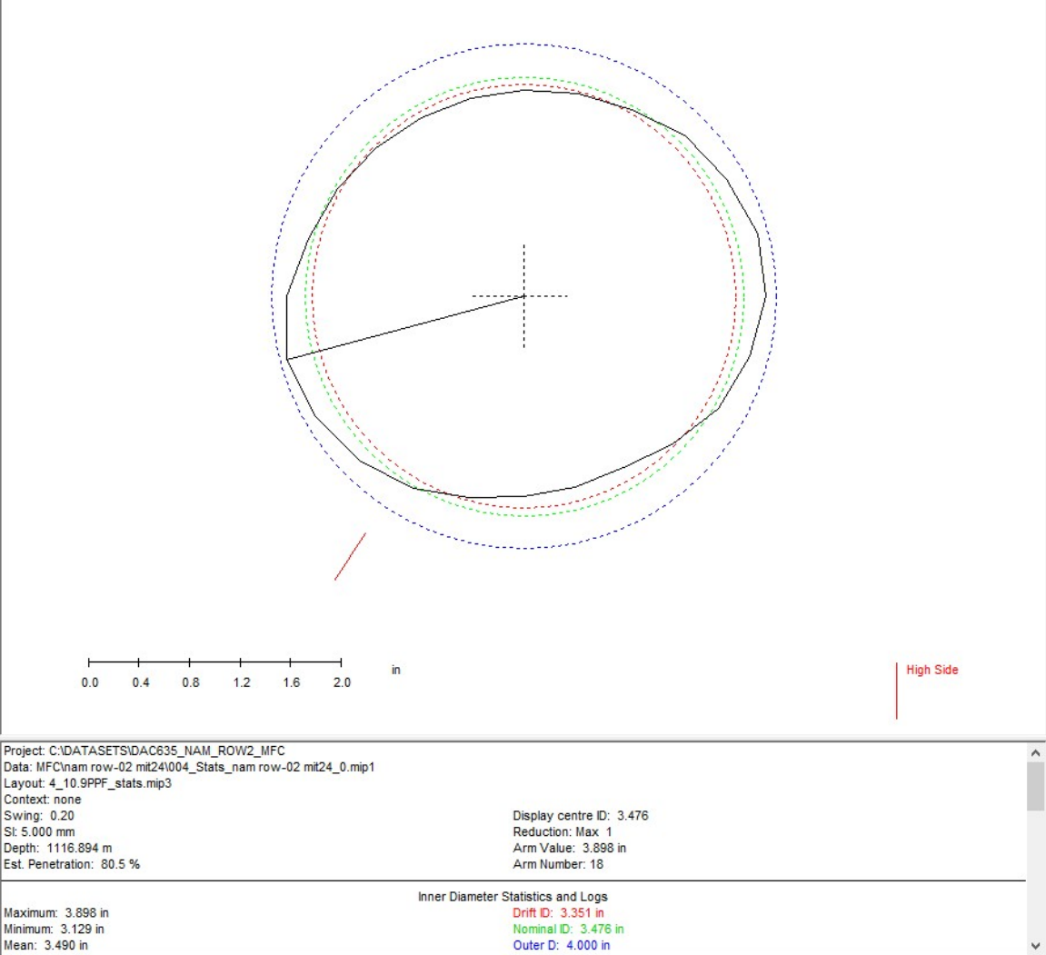
Figure 6: Maximum Recorded ID within 4", 10.9 lb/ft Tubing (Cross-section)
